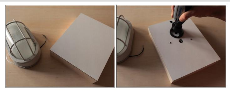
• Using your rotary tool, cut a hole in the cradled panel for the light fixture's wires and pull the wires through to the back.
